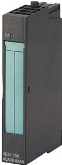
SIMATIC DP, ELECTRONIC MODULE ET200S: 2AI HIGH SPEED I-2WIRE, 0 - 20MA, 4 - 20MA, 15BIT, 15 MM WIDTH, FOR 2-WIRE TRANSDUCER, CYCLE TIME OF THE MOD.: 0.1MS, WITH LED SF (GROUP FAULT)
