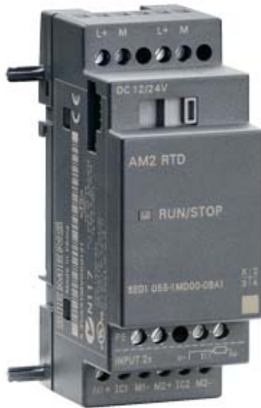
LOGO! AM2 RTD EXPAN. MODULE, PU: DC 12/24V, 2AI, -50 ... +200 DEGR/C PT100/1000
